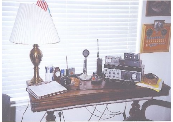
The loop tuning unit sits on top of the OMNI VI rig on the left side.
